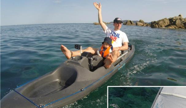
PEDAYAK Electric is a "hands-free" kayak with hybrid electric and/or muscular drive, manoeuvrable, stable, versatile and modular.
